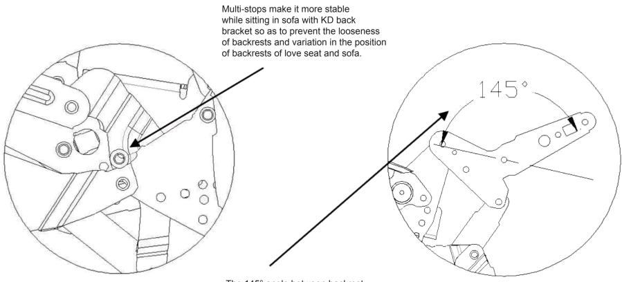
The 145° angle between backrest and seat box and the elevated footrest altogether help to realize best recline position with no stress on heart.
